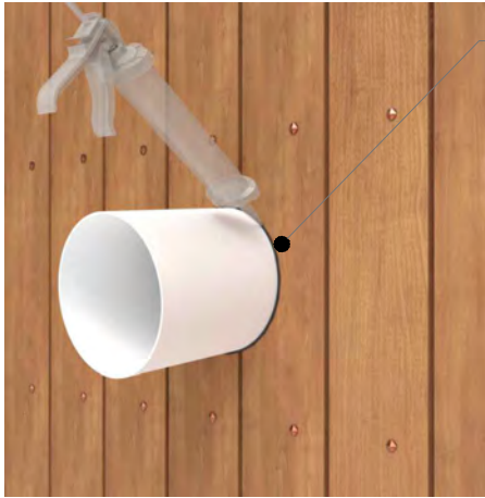
Continuous weather seal around pipe
