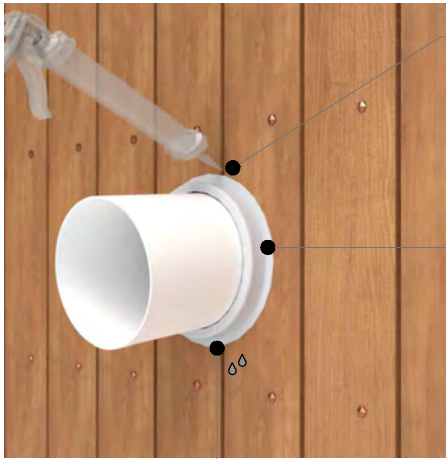
No sealant to drain
